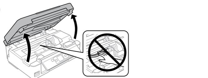
Open the scanner unit and press **OK**.
