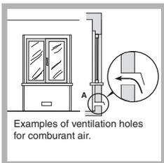
The air circulation system may take air directly from the outside by means of a pipe with an inner cross section of at least 100 cm<sup>2</sup>; the opening must not be vulnerable to any type of blockages.
