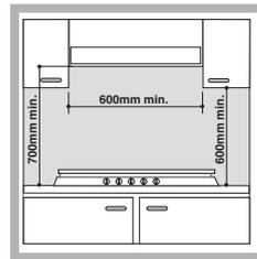
If the hob is installed beneath a wall cabinet, the latter must be situated at a minimum of 700 mm above the hob (*see figure*).
